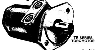
**TF SERIES TORQMOTOR** is for heavy-duty continuous applications that require up to 12 HP continuous with 20 HP peak. 4.9 CIPR to 29 CIPR, work PSI 49 to 18, 2000 PSI. Roller stator - 2 needle bearings in housing and 2 needle thrust bearings. Heavy back cover with 7 bolts
